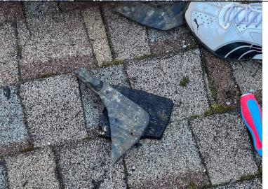
Photograph 15: Asphaltic membrane with a polyethylene surfacing.
